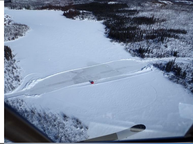
Photo #13: One section of the winter road at a lake crossing. An emergency shelter is present on the side of the road.
