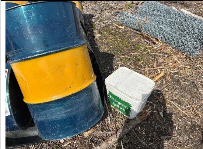
Photo #19: Sunmain fuel cache and a small spill kit which is not sufficient for the size of the fuel cache.
