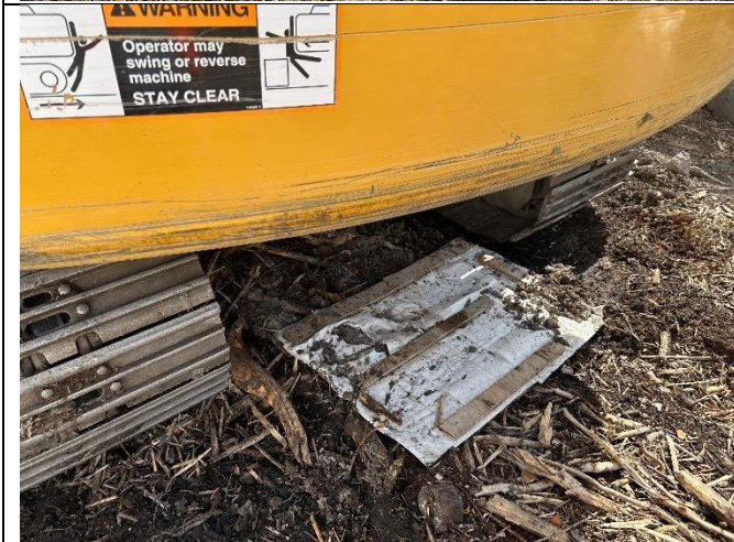
Photo #20: A drip tray appropriately placed under heavy machinery at Sunmain.
