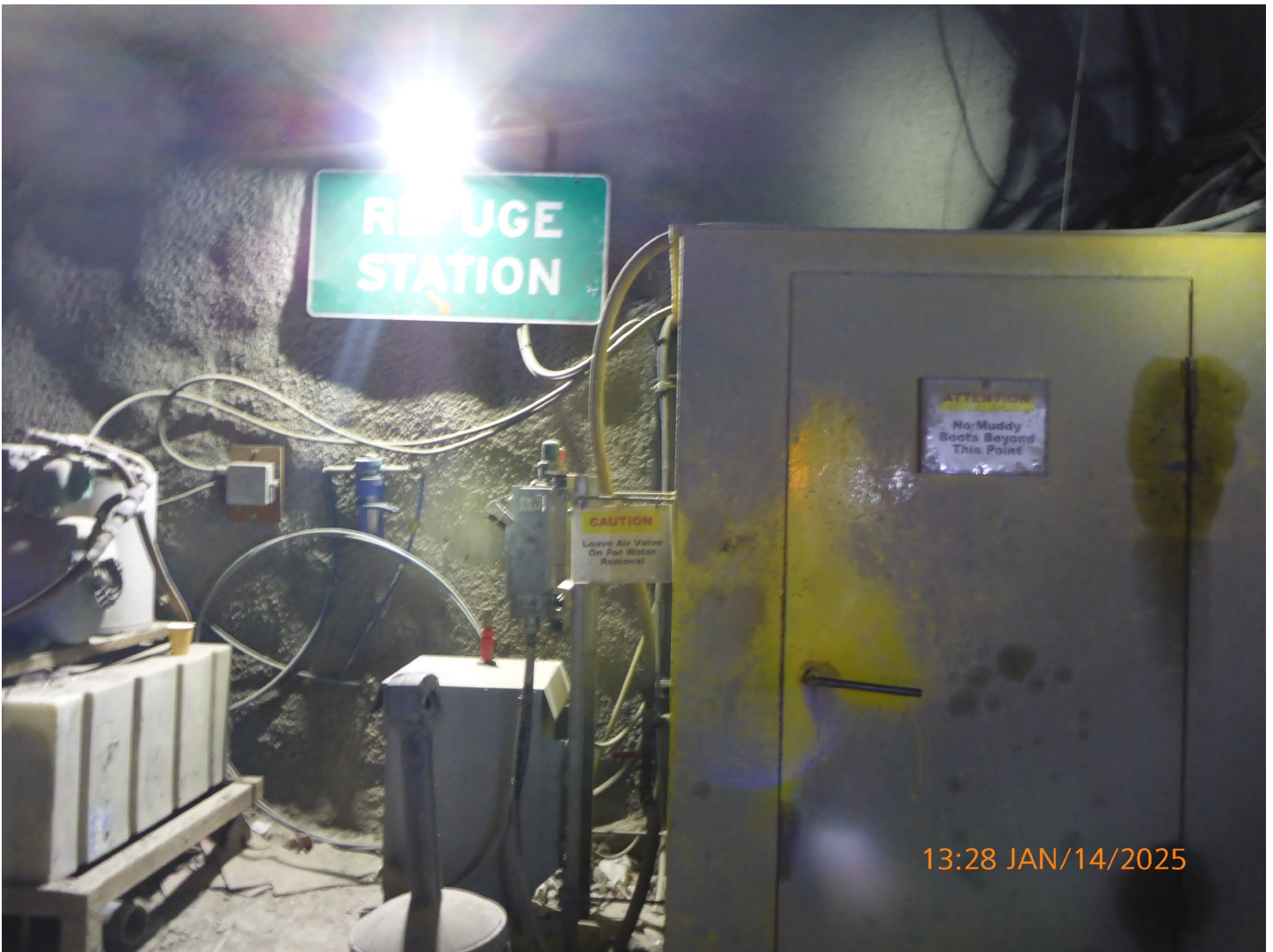
Photo 19 – Misery Underground – Refuge stations are located on strategic levels in the mine. The primary refuge station is used as a lunchroom for workers. The refuge stations were clean and maintained. Food waste is collected and brought to surface for disposal.
