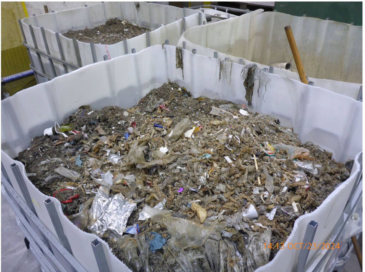
Photo 24 – Incinerator Building – Waste after it has been through the composter is dried out and rendered inert. It is then disposed of in the Landfill.
