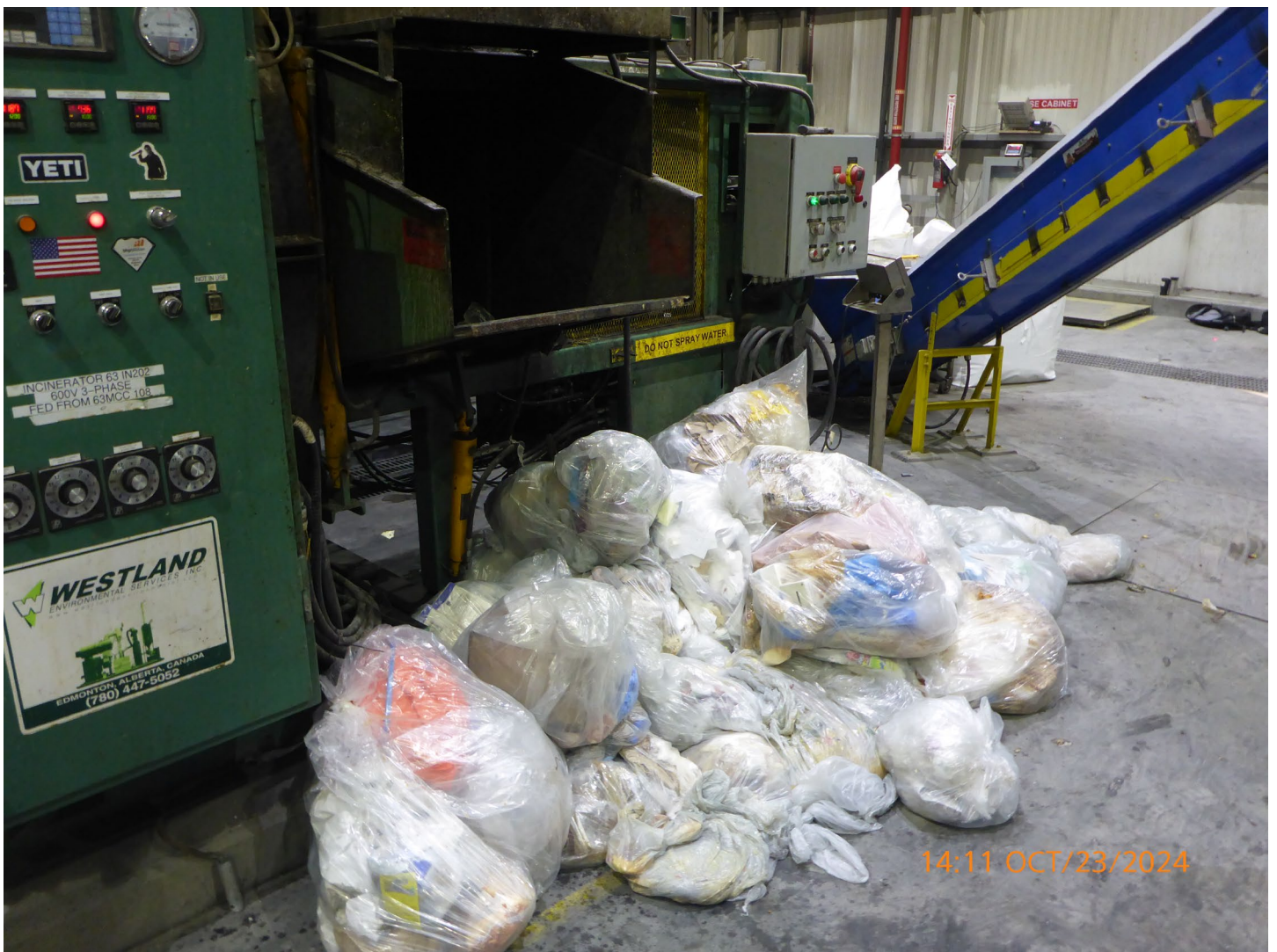
Photo 23 – Incinerator Building – Incinerator waste is segregated and batched. Much of the organics are sent to the composter, and the remaining waste is sent to the incinerators.
