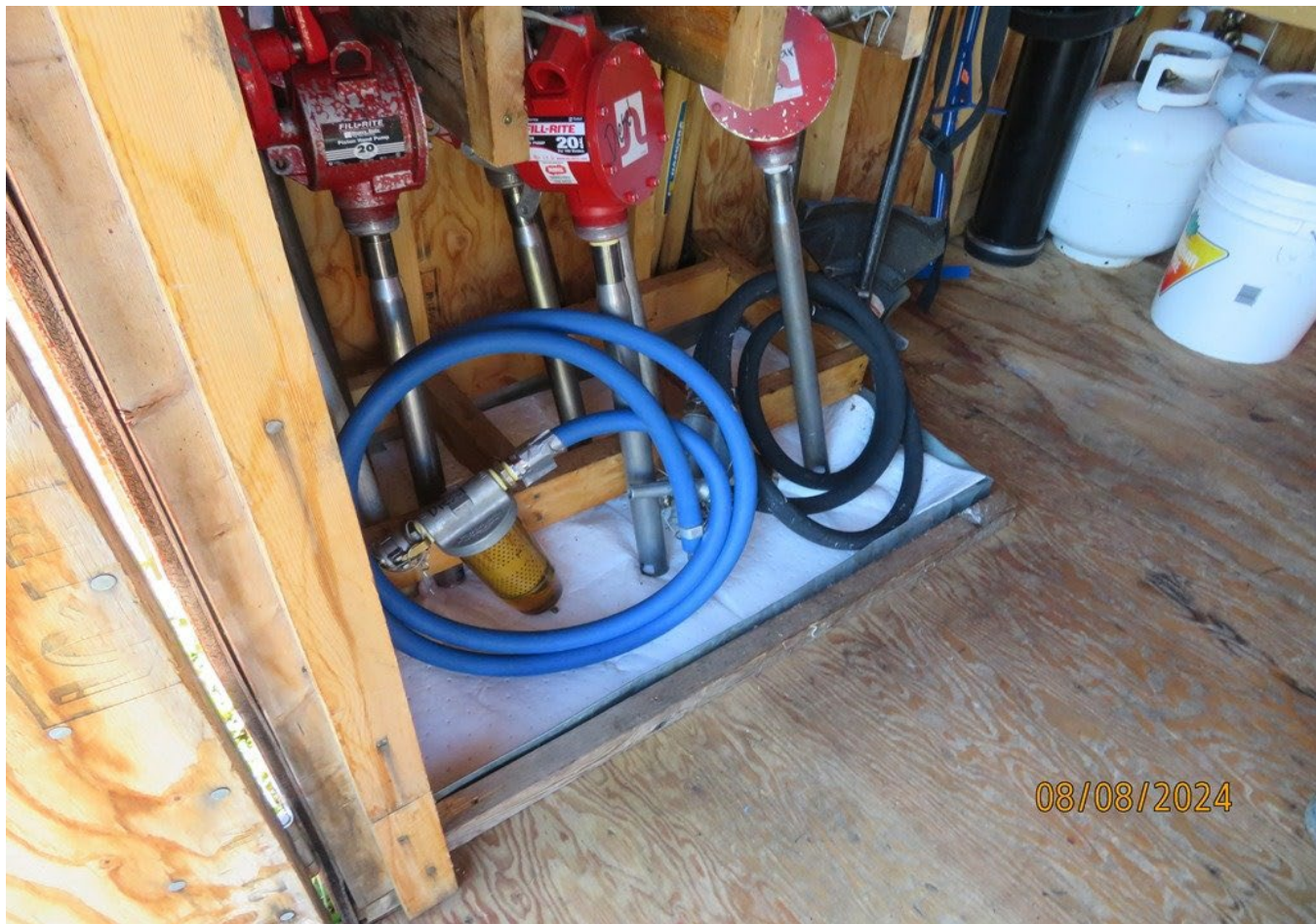
Figure 10 Absorbent pads and secondary containment are used where a possibility of leak is present.
